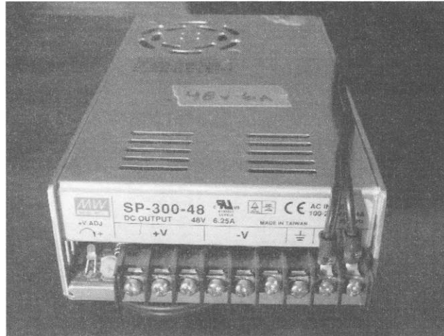
FIGURE 5-7 48-V 6-A power supply.
